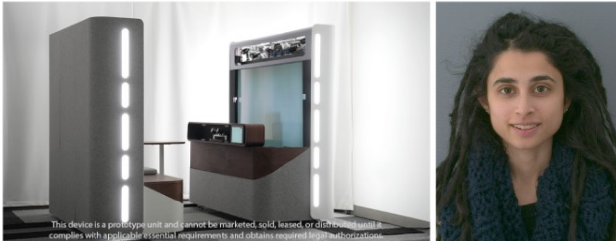
Fig. 7. Left: Our system prototype, showing the LED lights on the sides of the display and backlight units that create bounce lighting on the adjacent walls. Right: Illumination of a subject in our system.
