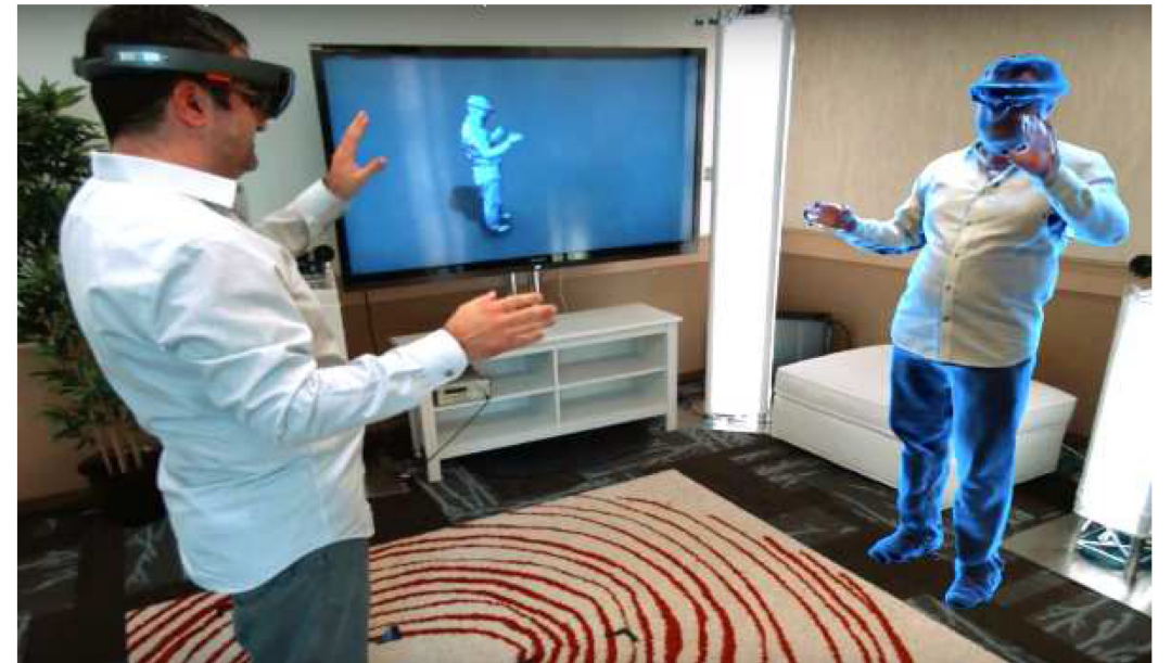
Figure 10.15: Holographic communication research from Microsoft in 2016. A 3D representation of a person is extracted in real time and superimposed in the world, as seen through augmented reality glasses (Hololens).
